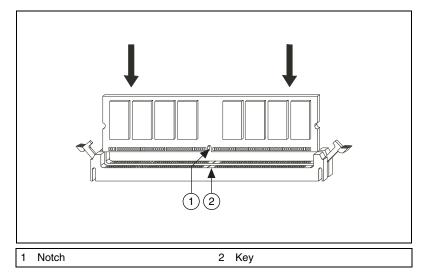
4. When the module is fully inserted, the plastic clip at each side of the slot automatically closes, as shown below.
